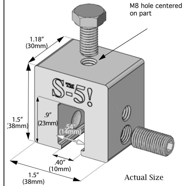
The S-5-U and S-5-U Mini clamps are each furnished with the hardware shown above. Each box also includes a bit tip for tightening setscrews using an electric screw gun. A structural aluminum attachment clamp, the S-5-U is compatible with most common metal roofing materials excluding copper. All included hardware is stainless steel. Please visit [www.S-5.com](http://www.S-5.com) for more information including CAD details, metallurgical compatibilities and specifications.
