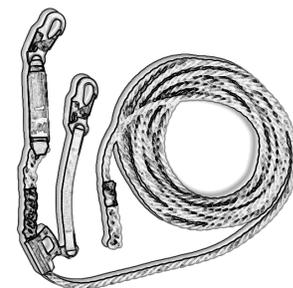
The shock absorber pack on the lifeline system, if your system has a shock absorber permanently attached to the end of the rope, is designed for attachment at the anchor point. If the shock absorber is built into the leg of the rope grab, positioning device, or fall arrester, that portion must be attached to the user's approved body harness.
