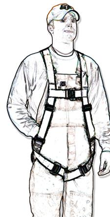
All buckles must be properly engaged and all straps must be properly adjusted before work takes place. Disengaged buckles, or improperly adjusted harnesses can cause severe damage in arresting a fall. Harness must not be worn excessively loose or the user risks significant injury even if the fall is arrested.
