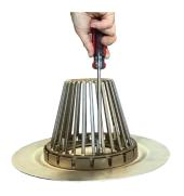
**STEP** Line up the three fastener holes on the OMG Vortex Breaker Strainer with the holes on the clamp ring and secure with the fasteners provided using a #2 square drive screwdriver.
