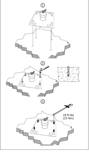
**3.5 INSTALLATION USING DBI/SALA TOGGLE BOLTS:** If the roof structure is at least 4 inches (10 cm) thick ("built-up" roof structure), the preferred method of installation of the Rooftop Anchor is with the use of DBI/SALA toggle bolts. The toggle bolts are designed to accommodate the maximum total roofing material thicknesses (including insulation and decking) listed below.
