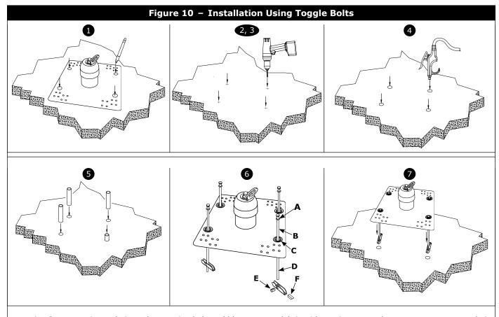
4. Insert an air nozzle in each mounting hole and blow out any debris with an air pump or low-pressure compressed air (Figure 10-4).
